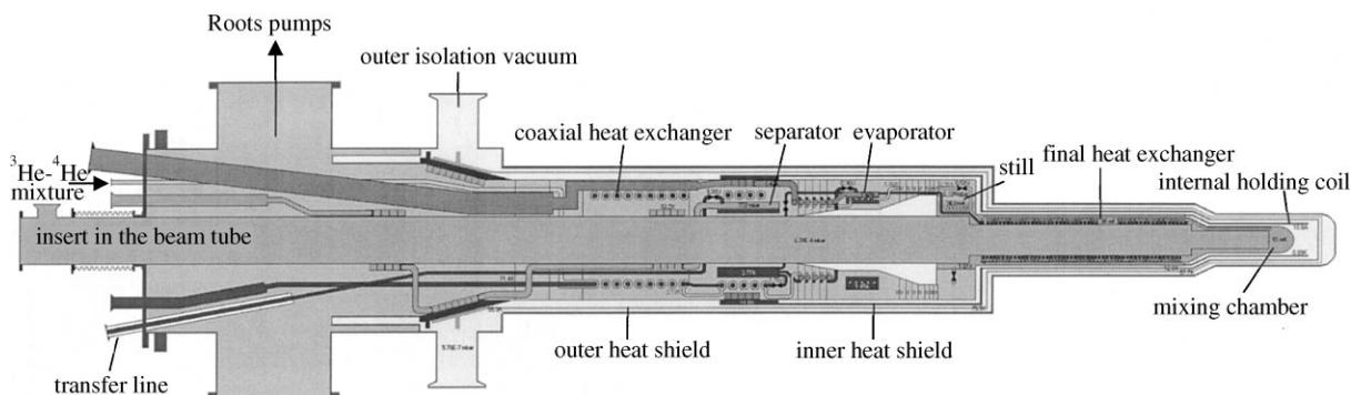
Fig. 4. Schematic diagram of the dilution refrigerator.
