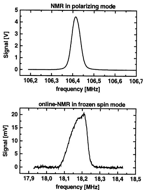
Fig. 10. Enhanced signals taken at 2.5 T using the polarizing magnet (upper diagram) and at 0.4 T using the internal holding coil (lower diagram).
