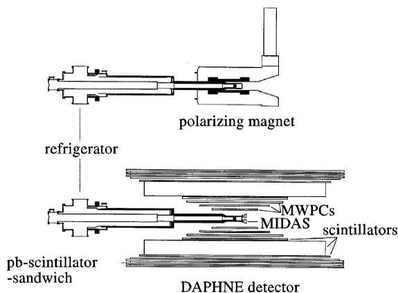
Fig. 2. Sketch of the refrigerator and the target area in the polarizing mode (upper sketch) and during the data taking in the frozen-spin mode (lower sketch).
