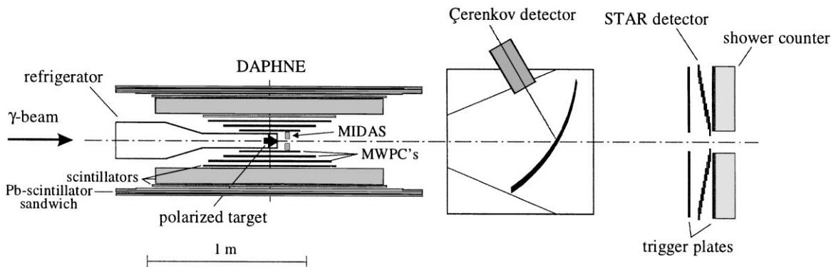
Fig. 1. Side-view of the experimental set-up at Mainz.
