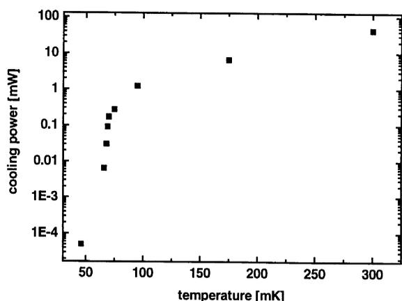
Fig. 3. Cooling power of the refrigerator.
