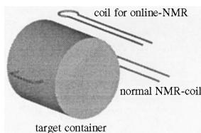
Fig. 8. Target container with the two NMR-coils.
