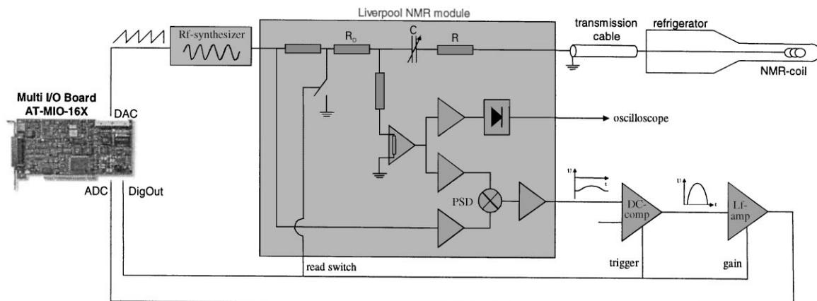
Fig. 7. Set-up for the NMR-measurement with the series Q-meter.
